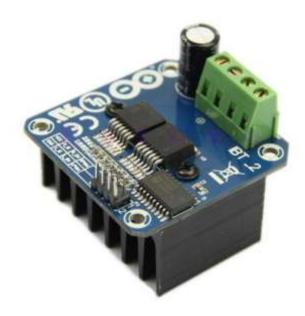
This driver uses two high current half bridge Infineon BTS 7960 chip for motor drive applications. Interfacing to a microcontroller is made easy using this driver which features current sensing, slew rate adjustment and protection against overn temperature, overvoltage, undern voltage, Overn current and short circuit.
