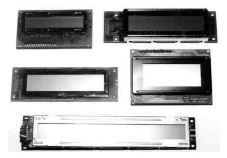
Several different liquid crystal technologies exist. "Supertwist" types, for example, offer improved contrast and viewing angle over the older "twisted nematic" types. Some modules are available with back-lighting, so that they can be viewed in dimly-lit conditions. The back-lighting may be either "electro-luminescent," requiring a high voltage inverter circuit, or simpler l.e.d. illumination.
