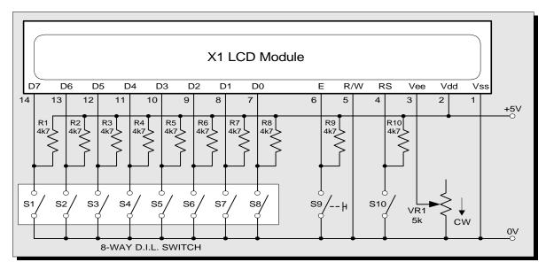
Figure 2: Circuit diagram for an l.c.d. experimental rig.
