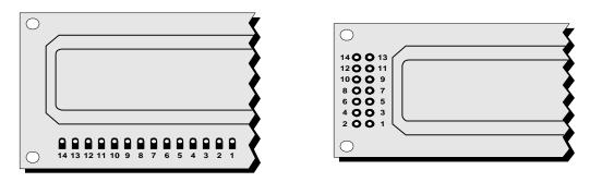
Figure 1: Pinouts of the two basic l.c.d formats.
