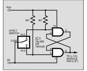
Note that the output of the "de-bounce" circuit is high when the switch is pressed and low when the
