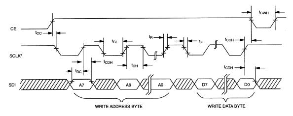
\*SCLK can be either polarity, timing shown for CPOL = 1.
