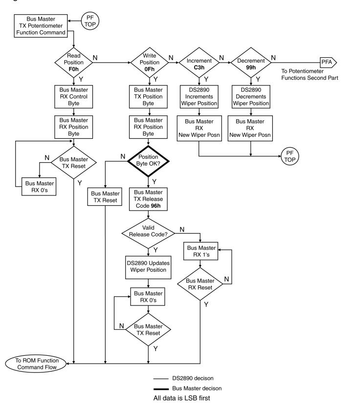
Figure 17. POTENTIOMETER FUNCTION COMMAND FLOW (continued)
