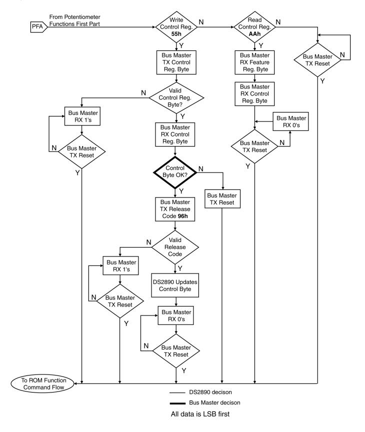
Figure 18. ROM FUNCTION COMMAND FLOW
