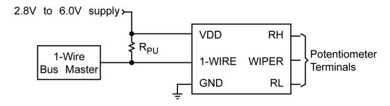
(a) Auxiliary V<sub>DD</sub> Supply Configuration
