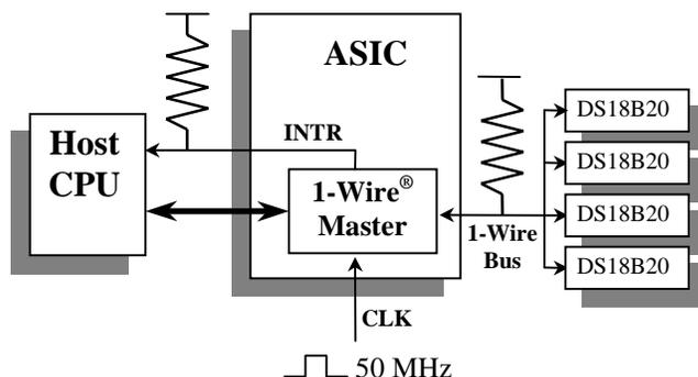
Figure 1 shows the circuit configuration this example will refer to. The 1-Wire Master has been designed into a customer ASIC and the host CPU will use it to order four thermal sensors to convert temperature and report their values. The 1-Wire bus and the INTR line each have a standard 5k pull-up resistor attached. A 50 MHz system clock drives the 1-Wire Master's timing through the CLK pin. The 1-Wire Master has been memory mapped into port address space of the CPU.
