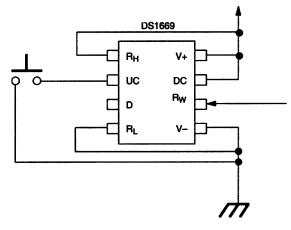
The DS1669 interprets input pulse widths as the means of controlling wiper movement. A single pulse input over the UC, DC, or D input terminals will cause the wiper position to move 1/64<sup>th</sup> of the total resistance. A transition from a high to low on these inputs is considered the beginning of pulse activity or contact closure. A single pulse is defined as being greater than 1 ms but lasting no longer than a second. This is shown is Figure 8a.
