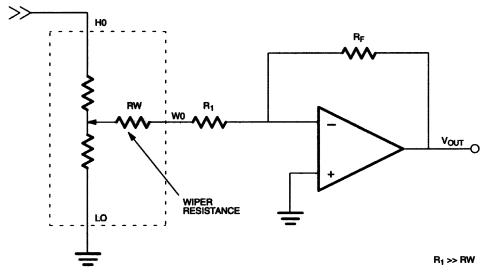
**INVERTING VARIABLE GAIN AMPLIFIER** Figure 9
