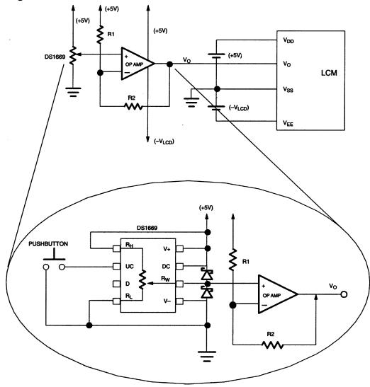
The output of the Op Amp drives the LCD contrast control voltage, V<sub>0</sub>, and is given by equation (1):
