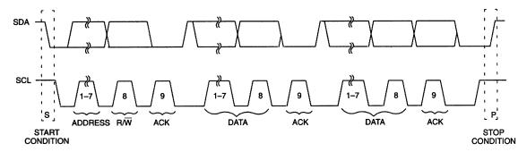
The master device generates all of the serial clock pulses and the START and STOP conditions. A transfer is ended with a STOP condition or with a repeated START condition. Since a repeated START condition is also the beginning of the next serial transfer, the bus will not be released. Data is transferred with the most significant bit (MSB) first.
