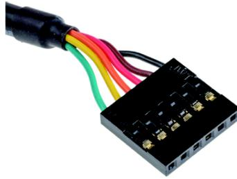
Figure 1.2: UART cable connector.
